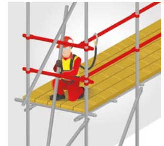
Figure 2: Always clip on when raising materials
