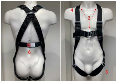
Figure 19: Correct Adjustment of Safety Harness
