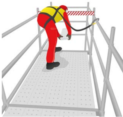
Figure 4: Leave a system deck in place to aid removal of others.
