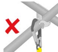
Figure 31: Transoms underslung on non-load-bearing couplers
