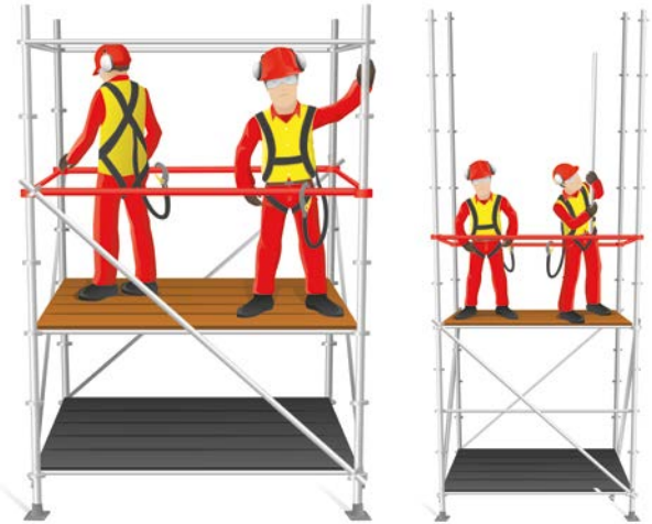
Figure 9: Short Lift Method
