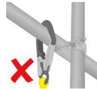
Figure 28: Ledger guardrail on single couplers
