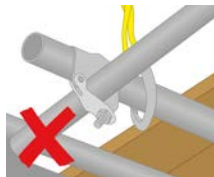
Figure 26: Transom below foot level
